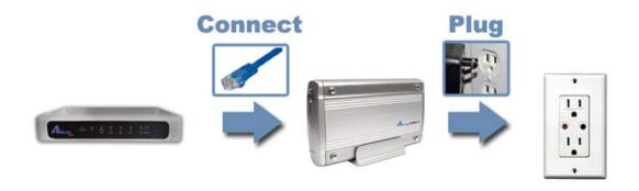
The Ethernet port on the HOMENAS is Auto-MDI/MDIX, which means you can connect it using either a crossover or a direct network cable.
